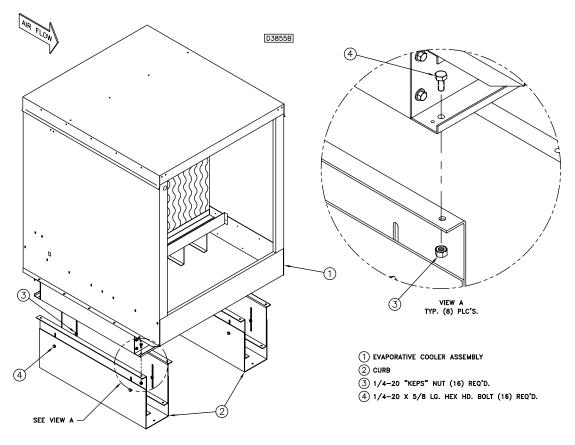
EVAPORATIVE COOLER CURB/PLATFORM MOUNTING ASSY 7-21-03
